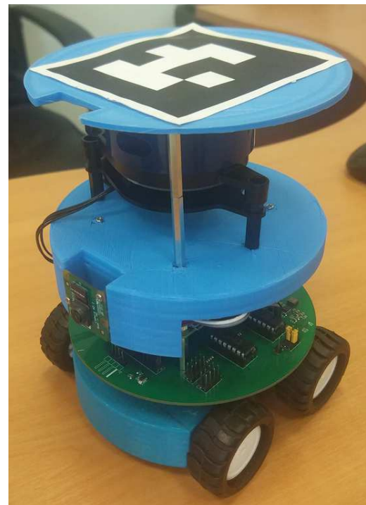
Fig. 6. The appearance of a prototype with a four-wheel chassis layout and an installed Lidar.
