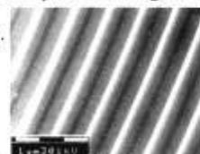
CGH pattern with 1.2  $\mu\text{m}$  spacing
